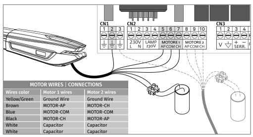
Connections should be made as shown above, connecting the 6 motor wires to the appropriate inputs of the central and capacitor.
