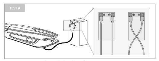
**Test A** • Make the connections as indicated in the image. If the motor works, the problem is in the control board. If it does not operate, do the test B.
