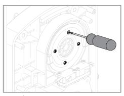
**03** - Slightly loosen the 4 screws of the magnetic actuator.
