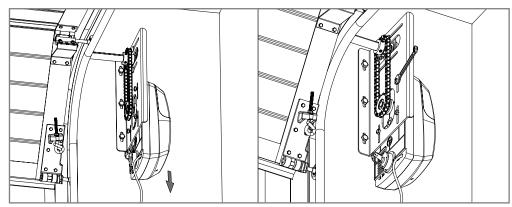
**08** - With the bolts still loose, pull the engine down in order to tighten the chain. While pulling down, fasten the 4 motor bolts to secure it on the support plate. The automatism is now installed.
