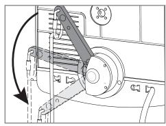
**08** - Lock the motor and test the door opening and closing using either the "PUSH" button on the control board or the transmitter. If necessary, repeat the previous steps, from the image 03, to better tune the limit switches.
