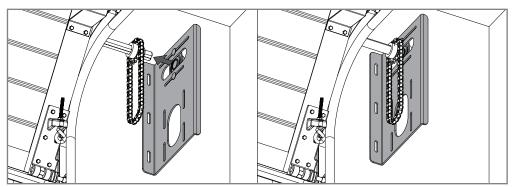
**03** - Pass the Ø25mm shaft through the bearing on the support plate.
