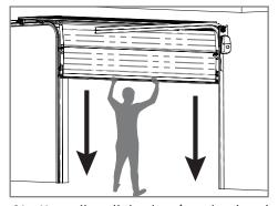
**04** - Manually pull the door into the closed position.
