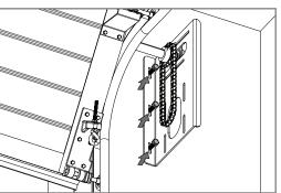
**05** - Pull the metal plate to the wall and secure with the screws.
