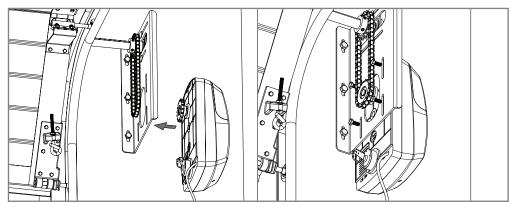
**07** - Place the automatism on the support plate (left), and assemble the chain on the motor's pinion as you can see on the right image.
