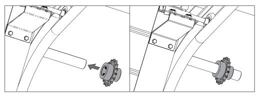
01 - Place the pinion on the  $\emptyset 25 mm$  spring's shaft of the sectional door.
