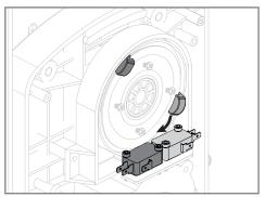
**07** - Move the plastic piece until hear a click from the micro. Now tighten the 4 screws of the magnetic actuator.
