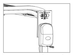
**02** - Open the automatism cover with a screwdriver and connect the motor to a power source at 230V.
