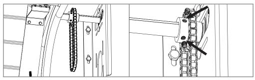
06 - Pull the pinion to the bearing and tighten the two bolts to secure the pinion to the shaft.
