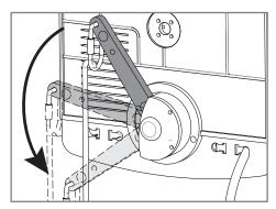
**01** - Unlock the motor, pulling the lever down. You will hear a little click when pulling down, and then you must let the lever go up.
