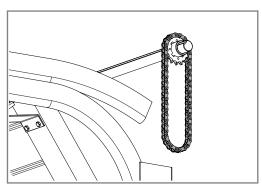
**02** - Place the chain over the pinion leaving it hanged.
