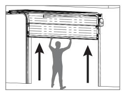
**06 -** Manually move the door to the open position.
